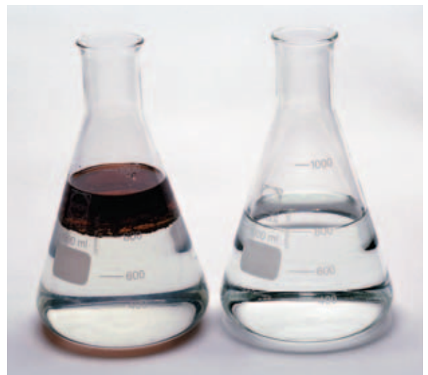
99% removal of oil in one single pass
